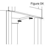
**Step 4:** Place spacer bar in Appliance Garage opening against Right End Panel. Position Left End Panel insuring, a snug fit against both shoulders of the spacer bar (See Figure 03).
