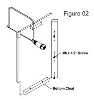
**Step 2:** If your countertop has a backsplash, the bottom rear corner of both end panels must be notched to fit over it. Measure and transfer the backsplash dimensions to each end panel. The bottom of the panel may be identified by cleats which are attached. Cut the notches with a fine-toothed coping saw. (See Figure 02) Then, notch the top of each panel to fit the bottom edge of the existing cabinet.
