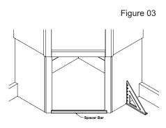
**Step 3:** Start three (3) #8x1/2" screws into pre-drilled holes (shown in Figure 02) in both end panels. Screw them in all the way and then back the screws out in the Right End Panel so that the Tambour Track will fit under the head of the screws. Take the screws all the way out in the Left End Panel. The screws will go in much easier later when you are working in the tight space inside the Appliance Garage.
