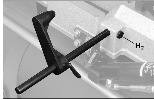
Figure 6-7: installing work stop (712V only)
