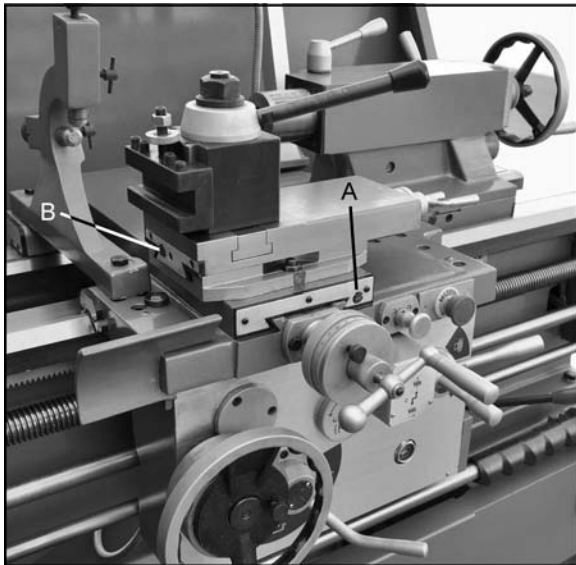
Figure 25 – Gib adjustments, slide and rest
