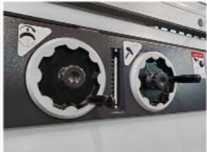
Main sawblade height adjustment and saw carriage tilt adjustment
