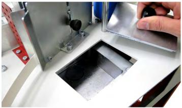
**Note:** The brand and quality of the glue is fundamental. Wurth recommends glues that work in the range of 130°C to 180°C.
