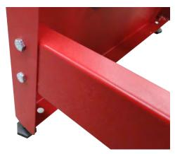
3. Place the adjustable hexagonal feet and position the machine upright on the floor. Set the positioning of the feet until the machine is level, then tighten the nuts next to the plate, as shown below:
