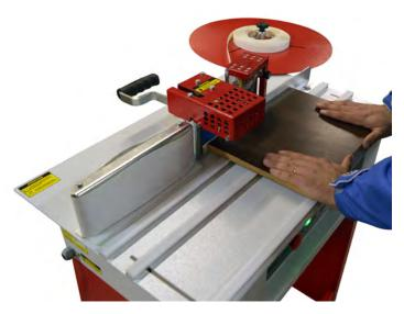
**CAUTION:** Crushing and cutting risk. Do not bring your hands within 10cm (4'') manual cutter. Do not wear loose clothing or gloves when operating this equipment.
