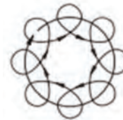
3/16" Orbit for general purpose sanding.
