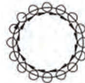
3/32" Orbit for fine finish sanding, less stock removal.
